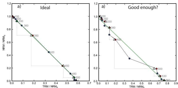
Figure 1: Examples of data from the paleointensity experiment. a) 'Ideal' results with straight-line behavior of the NRM/NRM<sub>0</sub> versus TRM/NRM<sub>0</sub>, where 'NRM' is the original magnetization and TRM is a laboratory induced magnetization. b) 'Non-ideal' results. (Figure modified from Shaar and Tauxe, 2013).
